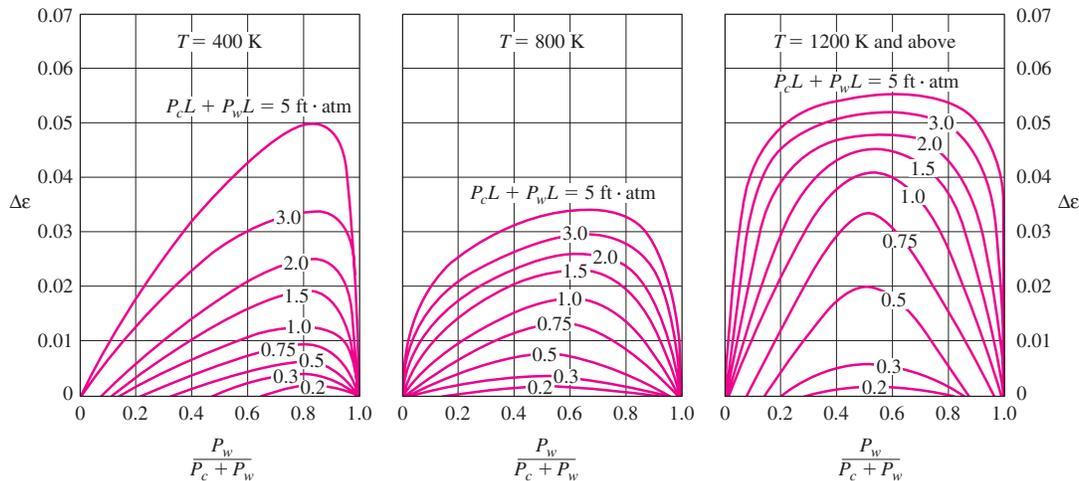
**FIGURE 12-38** Emissivity correction  $\Delta\epsilon$  for use in  $\epsilon_g = \epsilon_w + \epsilon_c - \Delta\epsilon$  when both  $\text{CO}_2$  and  $\text{H}_2\text{O}$  vapor are present in a gas mixture ( $1 \text{ m} \cdot \text{atm} = 328 \text{ ft} \cdot \text{atm}$ ) (from Hottel, 1954, Ref. 6).
