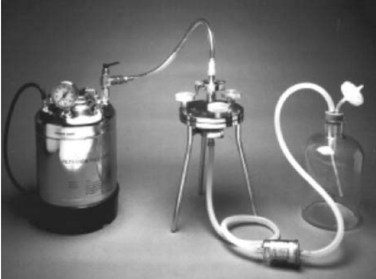
Figure 7.10 Sterile filtration of a small-volume pharmaceutical solution with a 142 mm plate-and-frame filter used as a prefilter in front of a small disposable cartridge final filter
